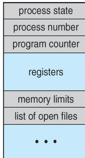
Figure 3.3 Process control block (PCB)
